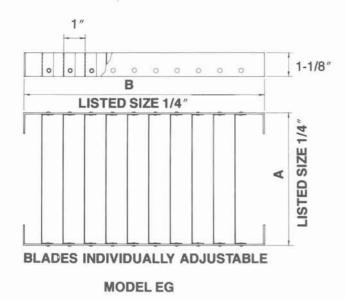
THE AIR-TRAC® MODEL EG IS DESIGNED TO STRAIGHTEN THE AIR FLOW GOING TO THE MAIN SUPPLY RUN.
