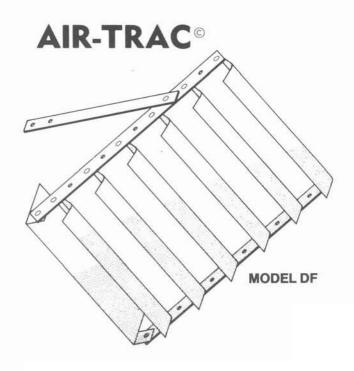
THE AIR-TRAC® MODEL DF IS DESIGNED TO EFFI-CIENTLY DEFLECT SUPPLY AIR INTO A BRANCH DUCT FROM A MAIN SUPPLY RUN. BLADES ARE INDIVIDUALLY ADJUSTABLE TO REQUIRED POSITION AND EACH UNIT IS FURNISHED WITH AN ADJUSTING STRAP. STANDARD MATERIAL IS GALVANIZED STEEL.
