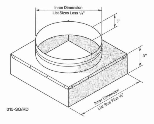
STANDARD CONSTRUCTION: • 28 gauge galvanized steel
